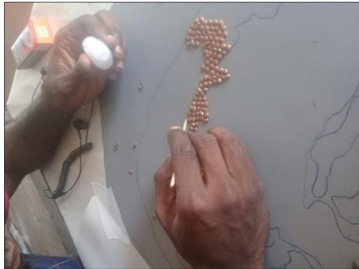
Fig 4: Copper domes placed by hand along a traced contour, using tweezers.
