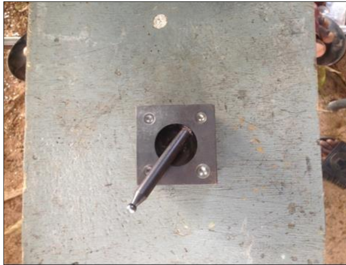
Fig 2: Doming block and punch used to raise flat discs into domes.
